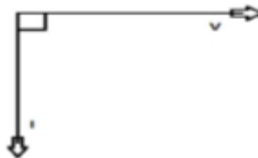
Figure 3: Current & Voltage 90° shifted
